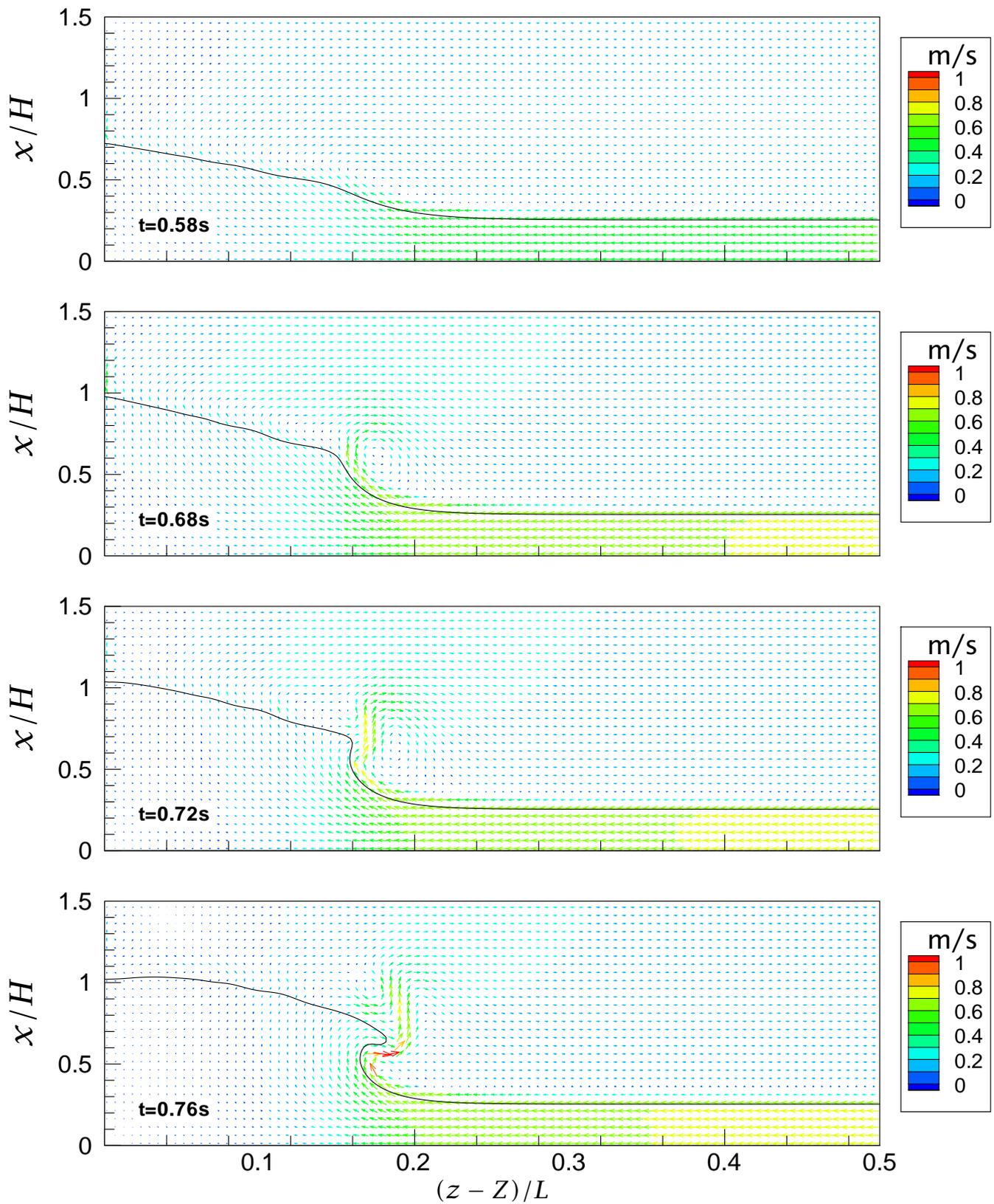
Velocity vector distributions obtained with PHOENICS (MUSCL scheme) for  $H = 5.08$  cm,  $f = 0.254$ , and the first piston acceleration law with  $\xi = 2$  and  $z_c = 0.5L$ .
