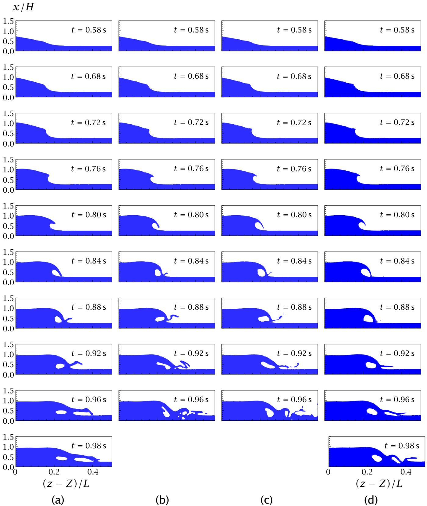
Wave profiles obtained for  $H = 5.08$  cm,  $f = 0.254$ , and the first piston acceleration law with  $\xi = 2$  and  $z_c = 0.5L$ . a) PHOENICS; hybrid scheme. b) PHOENICS; MUSCL scheme. c) Our code; reinitialization method of Sussman et al. (1998). d) Our code; method of Sussman et al. (1994) with local grid refinement.
