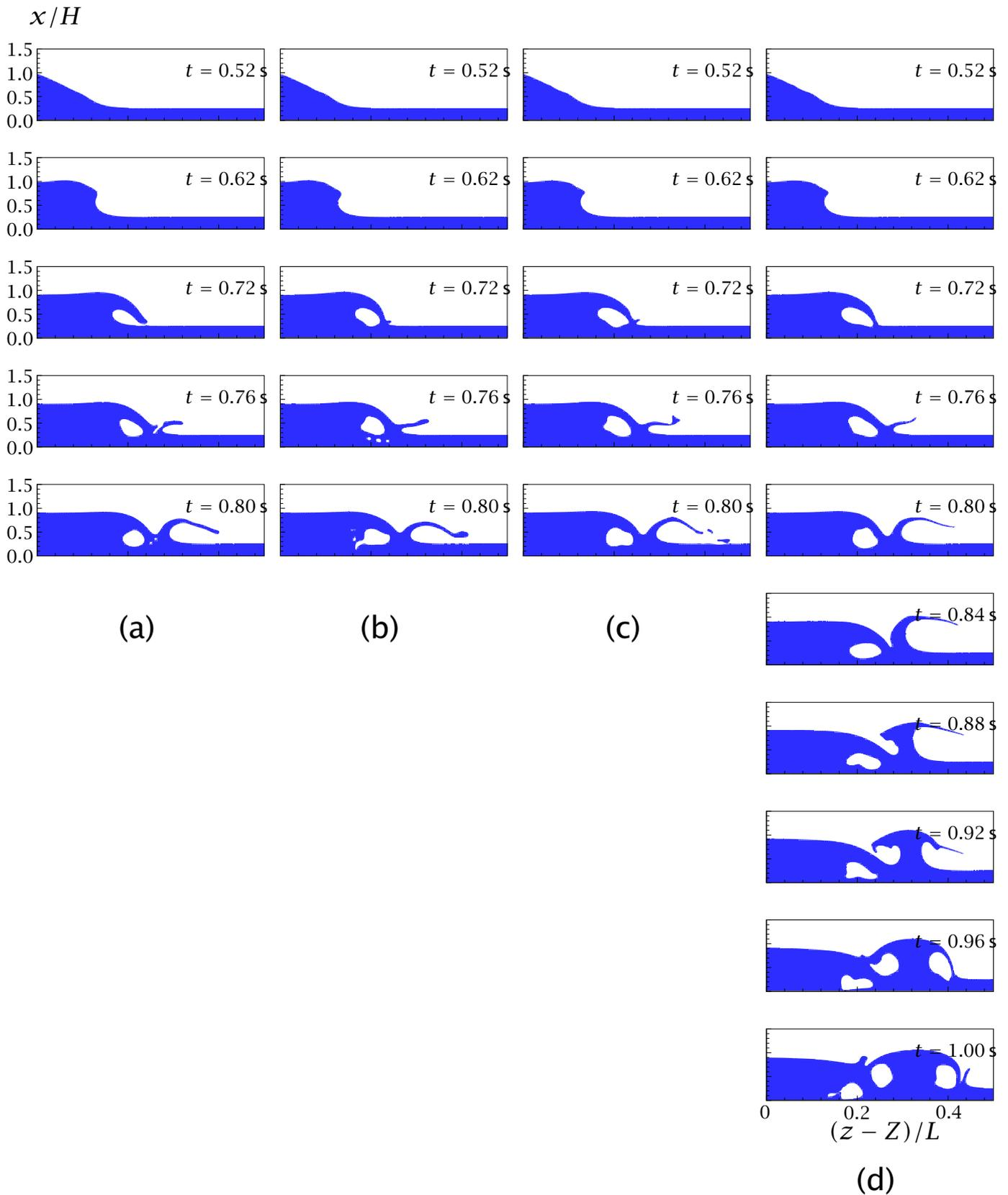
Wave profiles obtained for  $H = 5.08$  cm,  $f = 0.254$ , and the second piston acceleration law with  $\ell = 0.45L$  and  $t_H = 0.5$  s. a) PHOENICS; hybrid scheme. b) PHOENICS; MUSCL scheme. c) Our code; reinitialization method of Sussman et al. (1998). d) Our code; method of Sussman et al. (1994) with local grid refinement.
